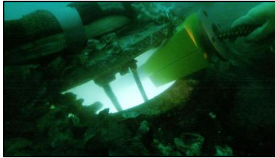
Figure 11 Drop camera illumination showing remaining hatch stirrup in place
