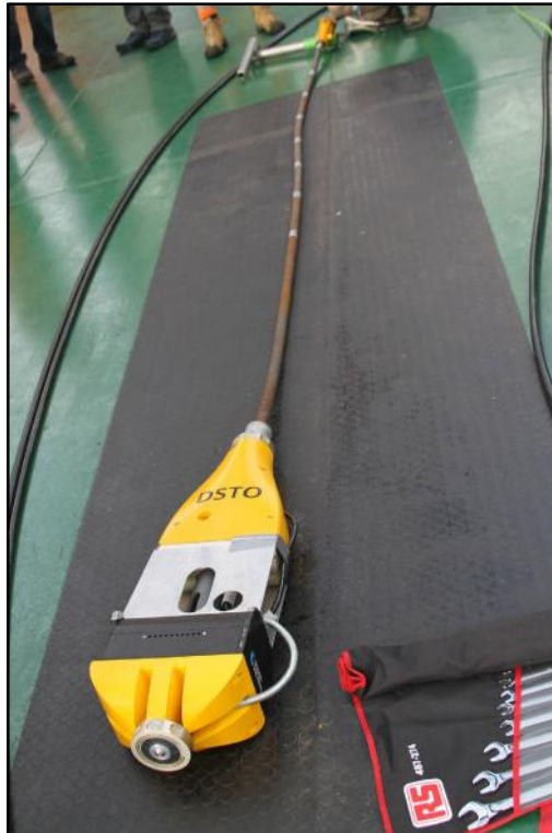
Figure 2 Modified Pole Camera with Aris Sonar Unit
