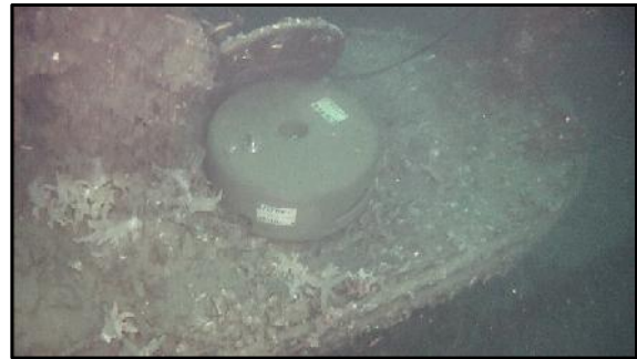
Figure 17 After anode pod after 48 hours of depletion; Hatch closure device (Top Hat) in place
