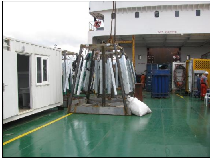
Figure 3: The three anode pods assembled on the deck of the dive support vessel.
