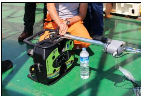
Figure 16 Spare ROV being used by the diver to rehearse using the 'boat hook' to extract the stuck ROV
