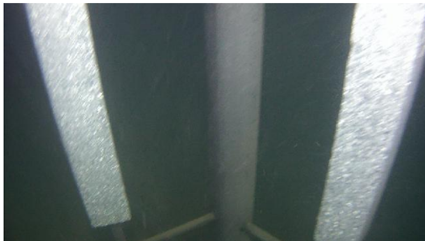
Figure 6: Corroding zinc anodes on the amidships pod two days after connection.
