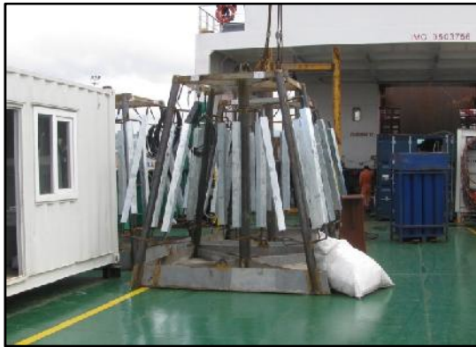
Figure 23 CPS Anode Pods; CPS Cable Connecting Clamp
